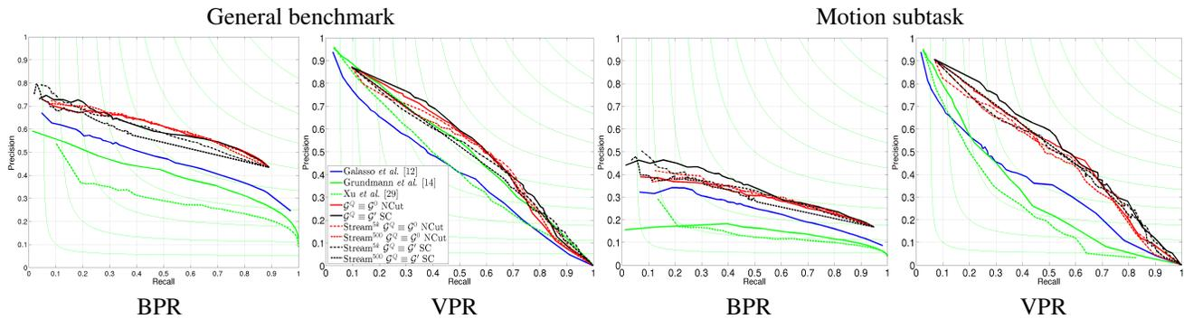
Figure 9. Evaluation of streaming algorithms with BPR and VPR on the general benchmark and the motion segmentation subtask of [13]. The proposed streaming variants (dashed/dotted red/black curves) of our graph reduction algorithms maintain performance and outperform video segmentation [14, 12] and streaming algorithms [29].
