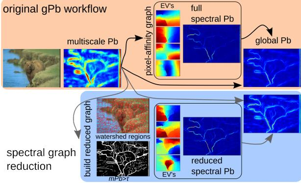
Figure 2. Workflow of [2] up to gPb. The computation of sPb on the pixel graph  $\mathcal{G}$  is replaced by computation in the reduced pixel-and-superpixel graph  $\mathcal{G}^Q$ . Superpixels are provided by watershed regions; in areas where  $(mPb) > \tau$  the grouping is considered uncertain and the single pixels are preserved as nodes. ( $\tau = 0$  means using pixels just, i.e. the original problem,  $\tau = 1$  means using only superpixels.)
